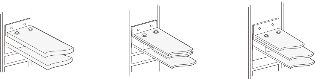
Figure 6.6-2 Recommended installation diagram of busbar
